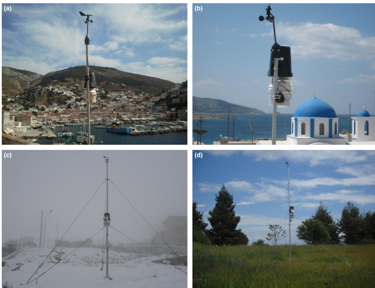
Figure 3. Examples of various setups of installed stations: (a) Hydra island, Saronic Gulf (port authority roof), (b) Koufonissi island, Southern Aegean (municipality office roof), (c) Arahova station, Central Greece (municipality water supply premises), and (d) Kryoneri, Peloponnisos (astronomical station).
